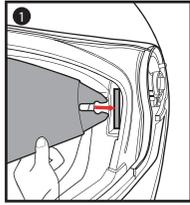
※When installing the sunlight film, be sure to have it slid behind the tap 'B' holder.
